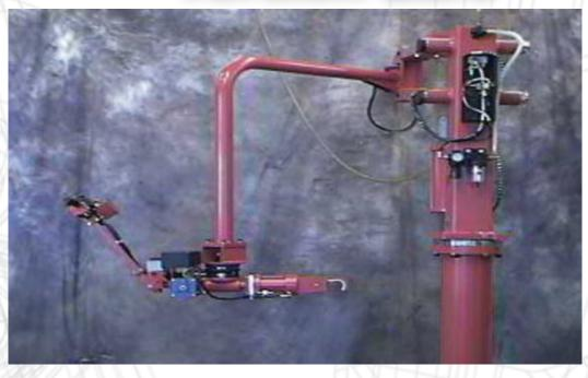
**Problem:** Existing hydraulic manipulator was not as effective at placing bars on the paint line hanger as a pneumatic manipulator would be. The "float" capability of a pneumatic manipulator and ease of maintenance convinced the customer to replace their hydraulic manipulator.
