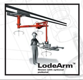
APPLICATION: Remove a mold hanging from an overhead conveyor, rotate it 180° with stops at 90° intervals.
