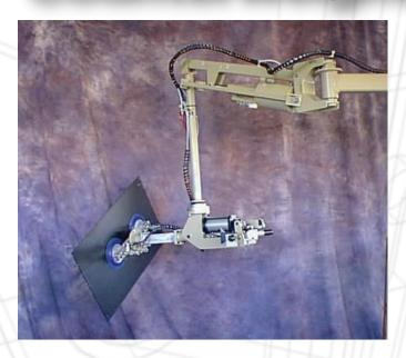
**Problem:** Lifting and inserting the counterweight, which may weigh up to 65 lbs., creates several ergonomic issues. There is a 10' dropped ceiling above the counterweight staging area. The opening in the cabinet is only 1" larger than the counterweight, which requires the pitched up counterweight be perfectly aligned for insertion. The cabinet is traversing the work cell moving by on a powered conveyor.
