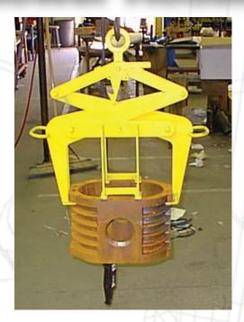
Problem: Various blower housing sizes and weights are to be handled with the same end-effector. After deburring, the blower housing must be placed onto a pallet in a specific orientation.
