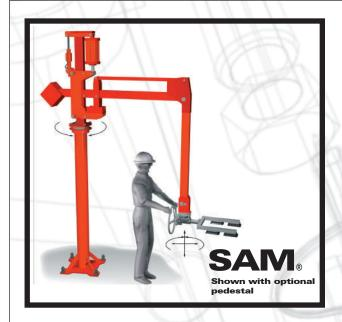
APPLICATION: Remove two cylinders from a customer supplied fixture which allows tool access. Transfer cylinders to the chassis, insert them into their mounting slots, and hold until the operator completes the installation.
