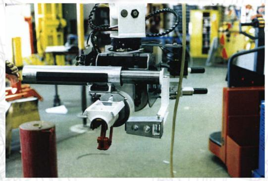
Problem: The vertical up and down dimensions of the manipulator end-effector was critical due to the large variation in roll heights and part orientations. The end-effector must prevent the rolls from telescoping when pitched down.
