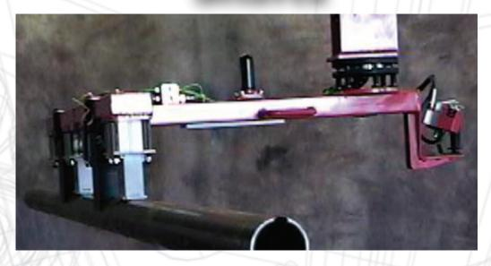
Problem: The core shafts are long and weigh 200 lbs. each. Two operators were required to handle the part. Finished drum surface couldn't be marred or scratched by the shaft. There were many work cell obstructions and limited floor space.
