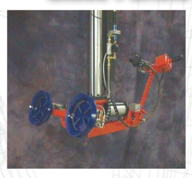
**Problem:** Safely pitch heavy glass panels varying in size, weighing up to 150 lbs. up to 110°, from vertical to horizontal and rotate through the pitched horizontal axis to line up holes for installation.
