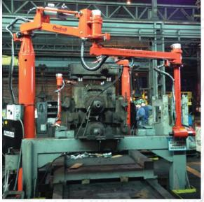
Problem: High torque application requiring 100 mm nuts being tightened and loosened on a steel fixture. The bolts were both in vertical and horizontal orientation. The application required the operator to use heavy impact wrenches, hand wrenches and sledge hammers. There was no ability to monitor the actual torque of the nuts and high potential for injury to the employee.
