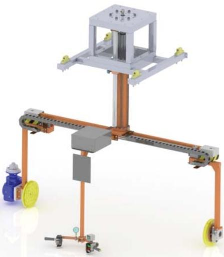
**APPLICATION:** Operators need to lift and flip small to large top chest and tool cases (tool boxes) on a conveyor to facilitate a downstream process. In some instances operators need to remove parts from conveyor and place on a work table then back to the conveyor.
