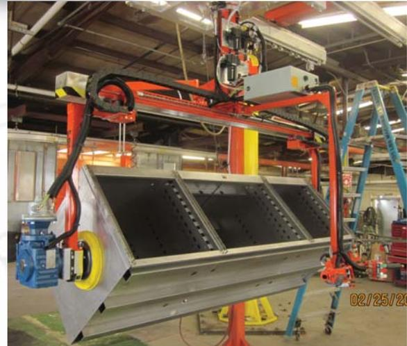
**Problem:** Parts range from 19.6-84" W x 15.5-26.8" H x 14.7-29.8" DP weighing up to 300 lbs. Process was requiring 2-3 associates to handle. The parts are coming straight from fabrication and may have some sharp edges and a thin oil film making handling them hazardous for the operators. Parts are partially assembled so operators need to be careful not to
