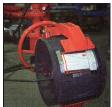
Tool grips and manually rotates a handling basket used for plating 250 pound parts
