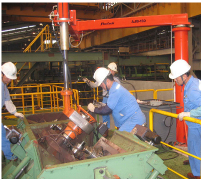
Pedestal mounted AJB with Vertical Lift Cylinder handling rotary dies.
