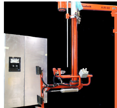
Pedestal mounted AJB with Vertical Lift Cylinder handling white goods.
